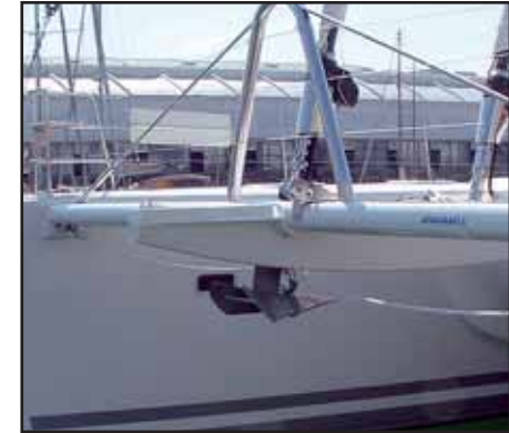
STROP INSIDE THE ANCHOR ROLLER
