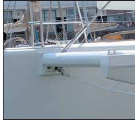
STROP FASTENING TO THE FORE BEAM
