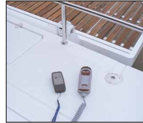
RADIOCONTROL + CONTROL OF THE DAVITS OR THE TENDERLIFT
