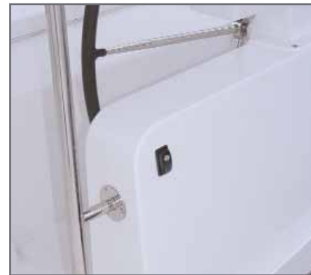
SWITCH (IN FLY) TO OPEN THE ACCESS HATCH TO THE FLY
