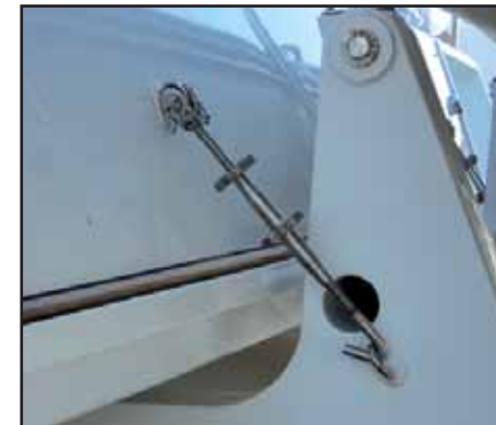
TURNBUCKLE OF THE TENDERLIFT
