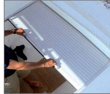
HAND OPENING OF THE 'ACCESS HATCH TO THE FLY
