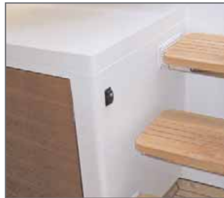
SWITCH (IN COCKPIT) TO OPEN THE ACCESS HATCH TO THE FLY
