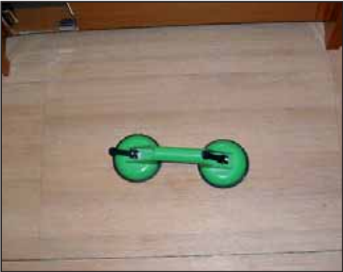
SUCTION PADS FOR THE FLOORBOARDS
