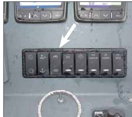
SYSTEM SWITCH FLYBRIDGE ACCESS LOCKING (ON THE FLYBRIDGE CONSOLE)
