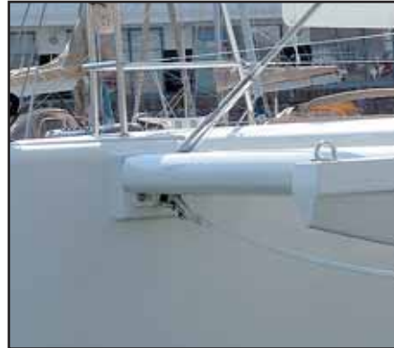
STROP FASTENING TO THE FORE BEAM
